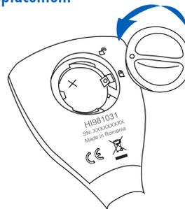
To change the CR2032 Li-ion battery, turn the battery cover located on the back of the meter counterclockwise to unlock. Remove cover and replace the battery with + side facing up.
