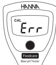
In calibration mode, if the meter displays an "Err" message when in the correct fresh buffer solution then the probe should be cleaned. Place the probe in the HI700682 cleaning solution for 20 minutes. Rinse with purified water and place in storage solution for 30 minutes before calibrating.
