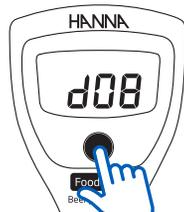
From measurement mode, press and hold the ON/OFF button. The meter will cycle through "OFF," "CAL," then current auto-off setting.
