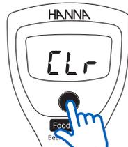
Place meter in calibration mode. Press and hold ON/OFF until "CLr" is displayed. The meter will now be at default calibration.
