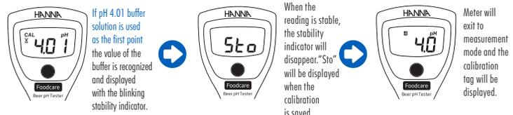
If pH 4.01 buffer solution is used as the first point the value of the buffer is recognized and displayed with the blinking stability indicator. When the reading is stable, the stability indicator will disappear. "Sto" will be displayed when the calibration is saved. Meter will exit to measurement mode and the calibration tag will be displayed.
