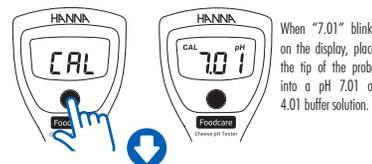
When "7.01" blinks on the display, place the tip of the probe into a pH 7.01 or 4.01 buffer solution.
