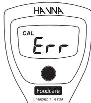
In calibration mode, if the meter displays an "Err" message when in the correct fresh buffer solution then the probe should be cleaned. Place the probe in the HI700642 cleaning solution for 20 minutes. Rinse with purified water and place in storage solution for a minimum of 30 minutes before calibrating.
