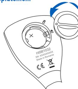
To change the CR2032 Li-ion battery, turn the battery cover located on the back of the meter counterclockwise to unlock. Remove cover and replace the battery with + side facing up.
