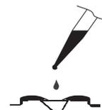
**Note:** If the temperature of the sample differs significantly from the temperature of the instrument, wait approximately 1 minute to allow thermal equilibration.
