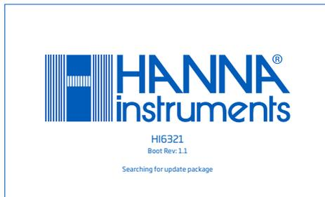
6. Wait for update to complete (~1 hour). **Note: Do not turn off the meter or disconnect from power.**
